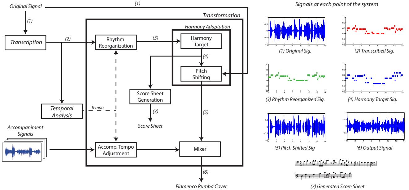
Figure 2: Block diagram of the Rumbator system. Emphasized blocks (in bold) correspond to transformation processes explained in Section 6
