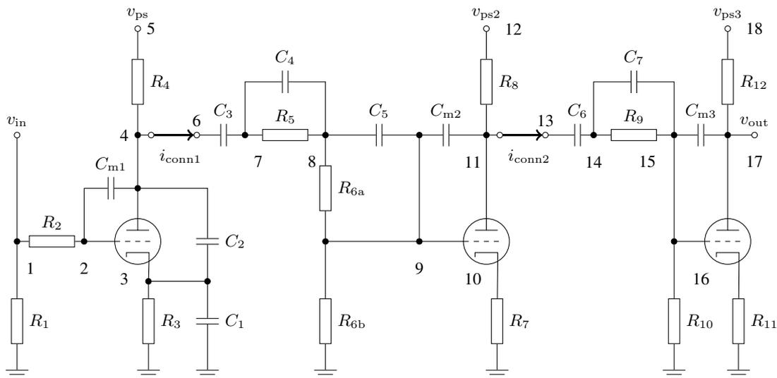
Figure 1: Circuit schematic of the Marshall JCM 800 guitar preamp with the decomposition into blocks. The blocks are connected using connection currents  $i_{\text{conn1}}$  and  $i_{\text{conn2}}$ .
