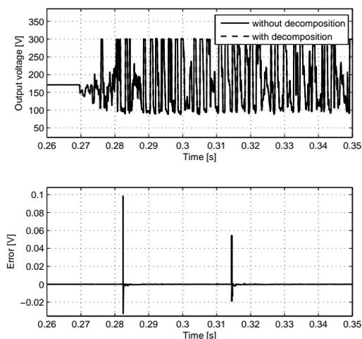
Figure 2: Comparison of output signals in time domain. The dashed line is overlapped with the solid and therefore their difference is also shown (bottom).
