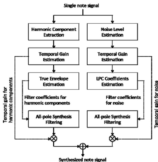
Figure 2: Harmonic plus noise source filter model overview.
