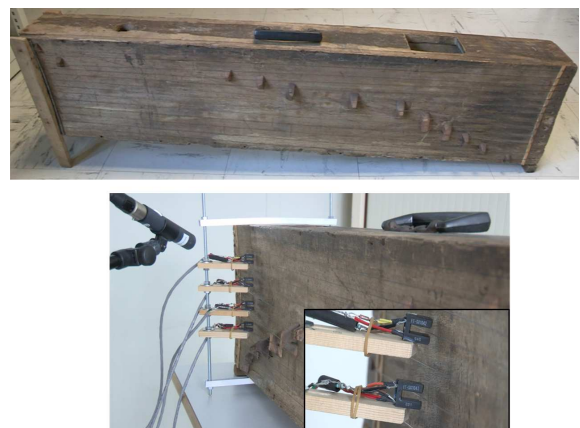
Figure 1: Photo of a zither marovany (on the top) and of the implemented optical-based system, with the details of sensors in the close-up (on the bottom)
